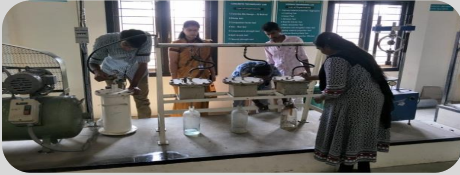
Permeability test of Concrete @ Structural Engineering Laboratory
