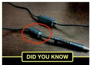
The little plastic thing at the end of Data Cables is called a Ferrite Bead and is used to block interference from radio signals from other electronics devices.
