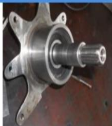
Fig.19 Oil seal for the gearbox along with clutch shaft
